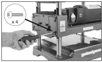
**Figure 9.** Cord wraps installed with #2 Phillips head screwdriver.
